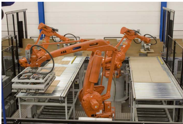
Figure 2. Two small robots work in one canter for cutting and handling based wood boards products.
