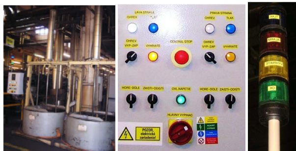
Figures 7: View of the machine after reconstruction, control panel and industry beacon (with Slovak labels)
